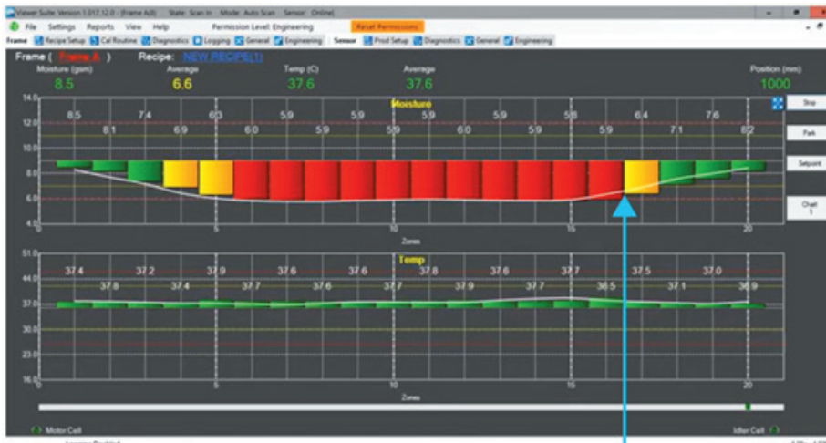
The white line indicates the moisture profile of the last scan
